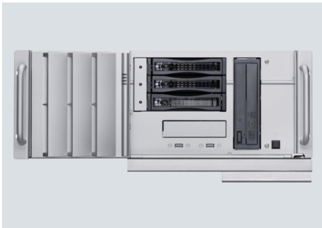
Front view of SIMATIC Rack IPC547D, with open front flap
